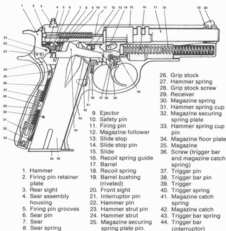
In the early model CZ 75 pistols, there was no half-cock notch to hold the hammer away from the firing pin (I), thus making an accidental discharge possible when the hammer was struck.
