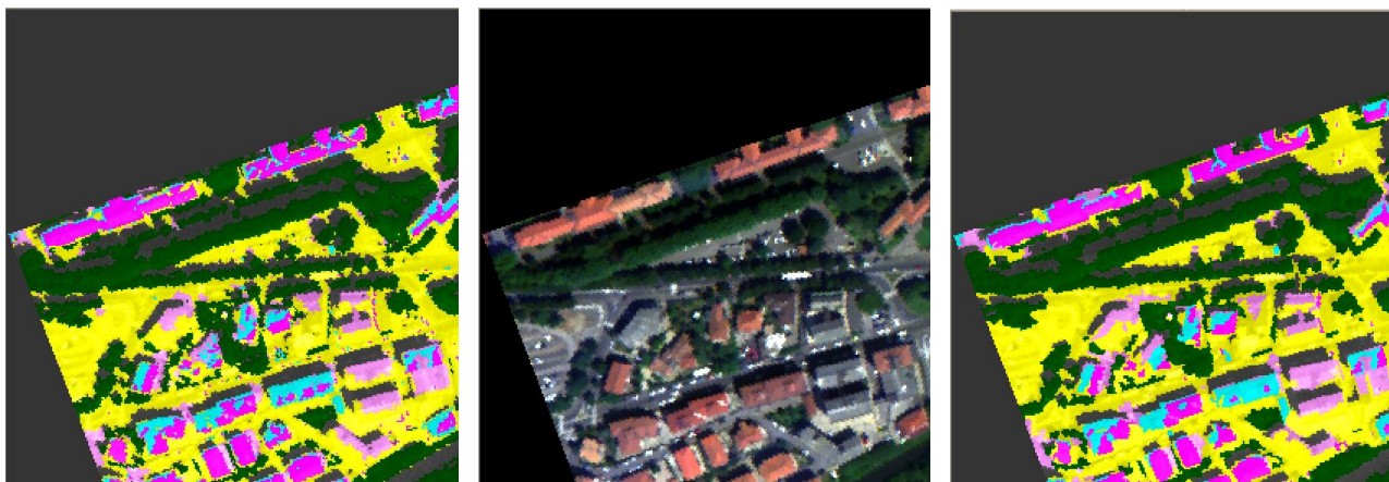
Fig. 7 Fuzzy method results applied to segmentation with scale factor 10 (on the left) and 40 (on the right) in the center a portion of the original ROSIS image.
